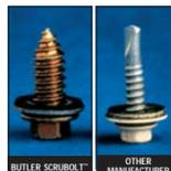
and panel attachments. In addition to providing a weak structure, self-drilling leaves behind metal shavings, which ultimately create rust problems. Butler factory punches structurals, and we use the Butler Scrublot™ fastener for clip and panel attachment. The high-strength, substantial Scrublot fastener has twice the pullout strength of industry-standard self-drillers. It takes two to three times the number of self-drilling screws to equal the performance of one Scrublot.
